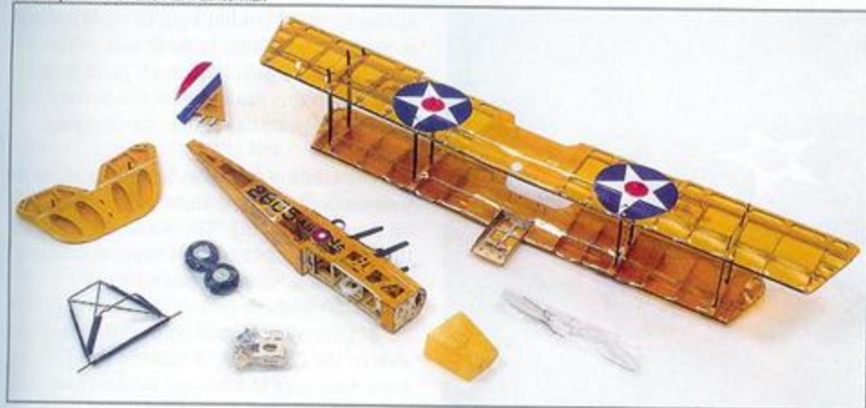
Notice the carbon-fiber LE and turtledeck spine. The hardware package has matching covering for repairs.
