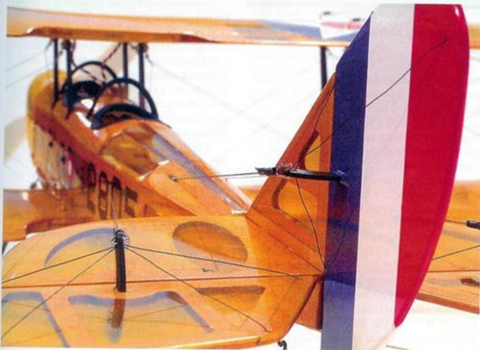
The control surfaces are installed at the factory with film covering for hinges. The pull-pull control matches that of the full-scale aircraft.
