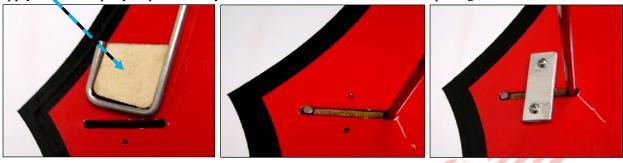
e. Position each fiberglass wheel pant at 90-degrees to the wing, then lower the wheel pant over its maingear strut toward the wing's surface.
