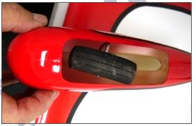
g. Position each wheel pant so its wheel has equal side-to-side clearance. Using three predrilled holes in each wheel pant and three wood screws, secure each wheel pant to its wing panel.
