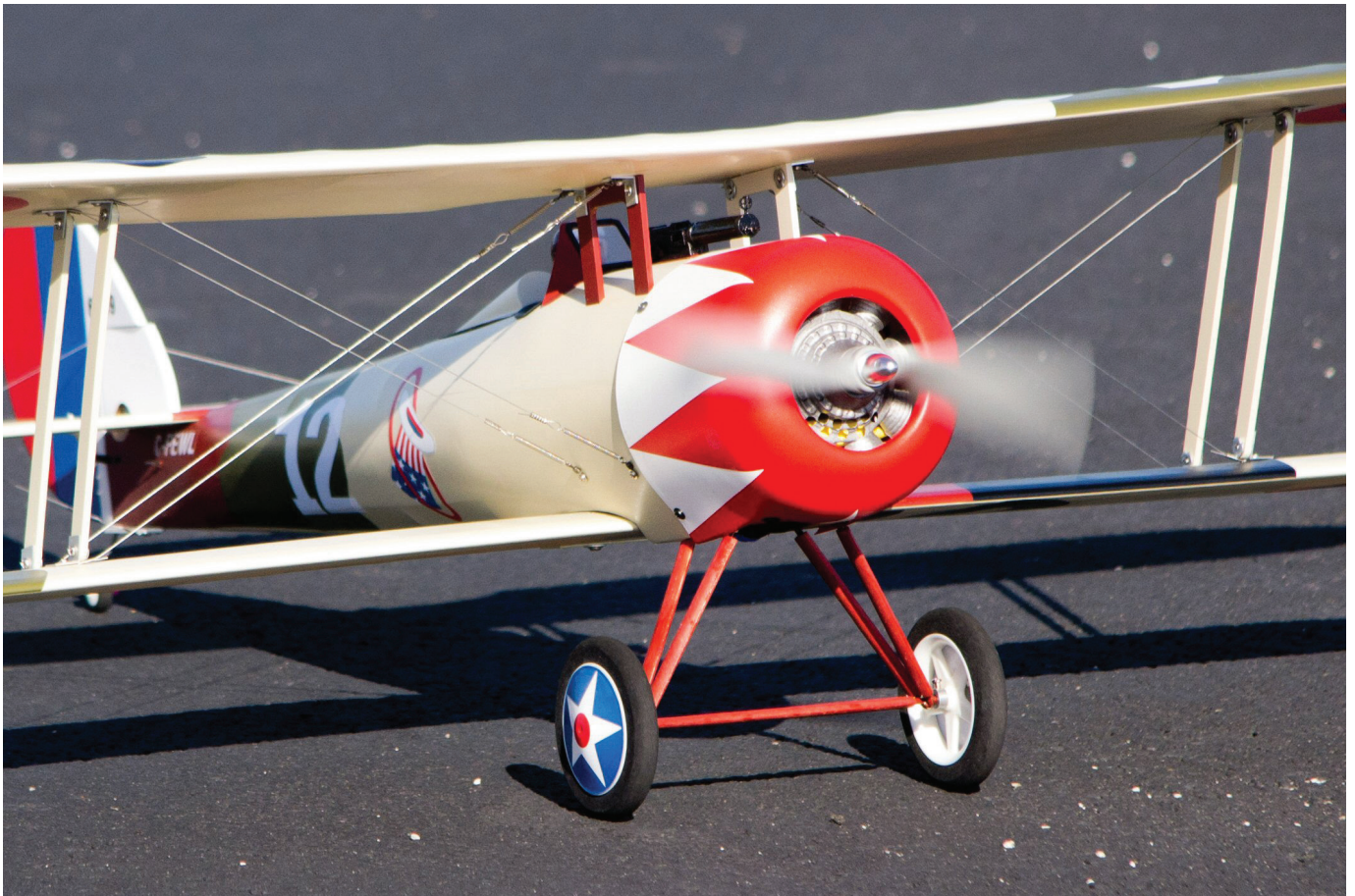
The 40-inch wingspan Nieuport 28 has an impressive list of detail features, which is unusual for this size model.
