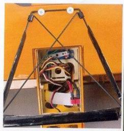
The preassembled landing gear is held on with four nylon bolts (two shown). The battery was placed just forward of the white hook and eye piece, and this battery/radio access area is covered with a spring-tab hatch.
