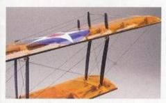
The wings, struts and flying wires come fully assembled. The nuts are not fully tightened, and all you have to do is raise the top wing to the correct height, and all the wires become taut—a tremendous construction time-saver.
