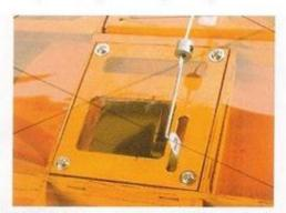
I like to have some leeway in adjusting control-rod lengths and opted for this arrangement, rather than a Z-bend on one end and a 90-degree bend on the other (which is how the instructions say to make the aileron control rods).
