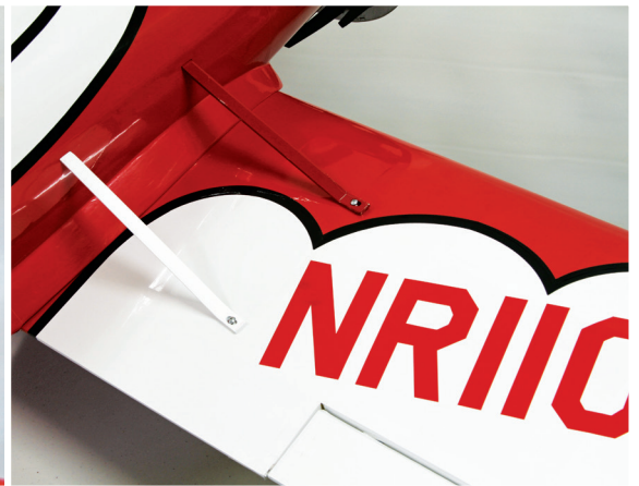
The outer ends of the strut are attached by drilling hard points on the wing.
