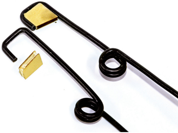
The addendum to the instruction manual addressed modifying the landing gear blocks to fit the new wires.
