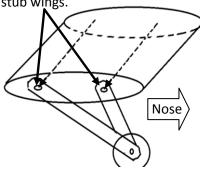
3. Test-fit the strut attachment bolts, landing gear struts and nuts.
