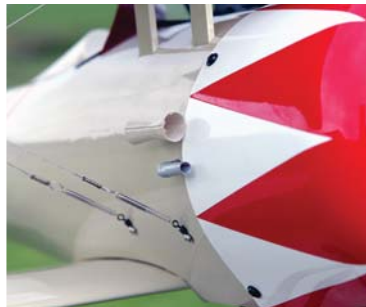
The fiberglass cowl comes pre-painted and the 9-cylinder dummy Gnome is pre-glued into place. Note the air intake and venturi on the starboard side.
