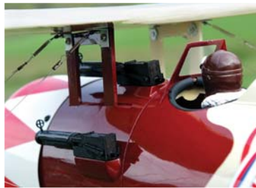
The two machine guns mount on curved plastic piece that is glued to the top, middle of the cockpit. The forward edges of the molded blocks in the plastic part align with the leading edge of the aft cabane strut.
