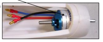
4. Use the supplied metal mounting plate and the hardware provided with your motor to install the motor in the nose as shown.
